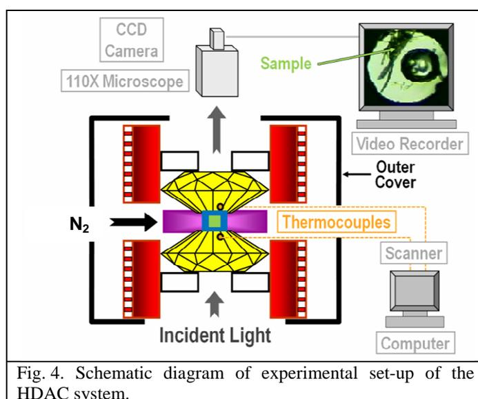
Fig. 4. Schematic diagram of experimental set-up of the HDAC system.
